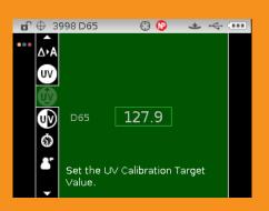
Calibrated UV component – first X-Rite handheld spectrophotometer with adjustable UV component to fully characterize optically brightened
